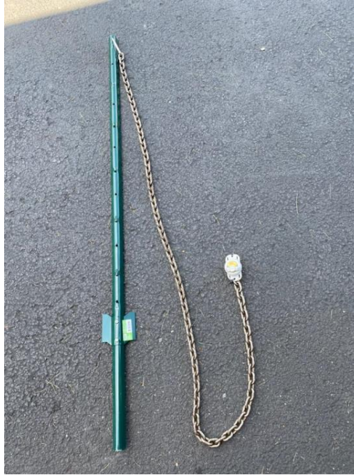
Figure 13 Stake & chain deployment apparatus for KLO stations.
