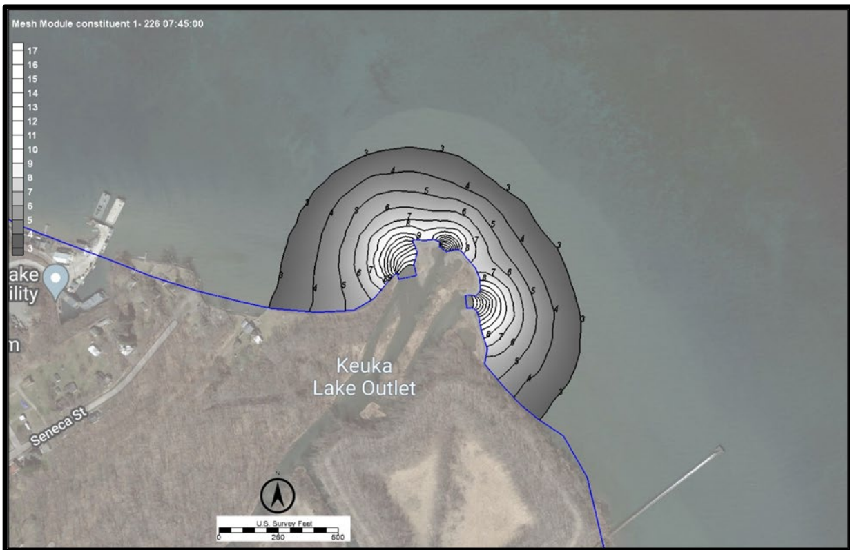
Figure 6.4: \Delta T Contours for Scenario Simulation 2 at 8/14/21 07:45. The enclosed area where \Delta T is \geq 3^\circ\text{F} is 16.4 Acres
