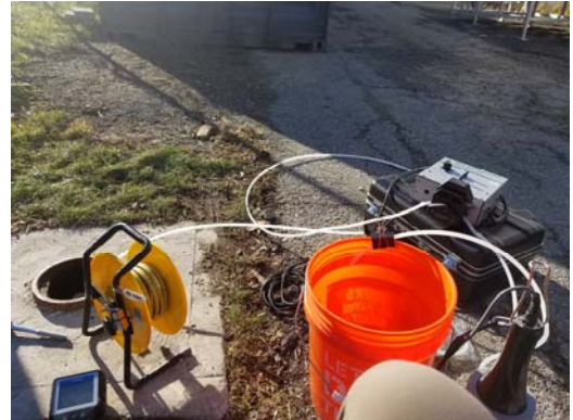
Photo 2.5: Typical groundwater sampling setup.
