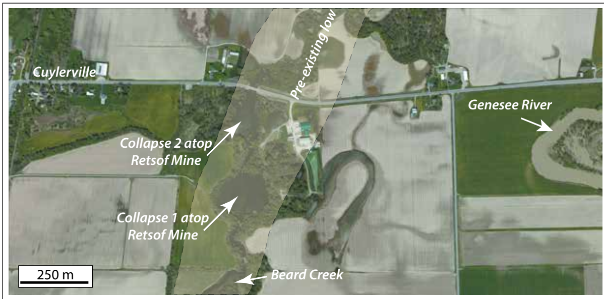
Figure 13. Location of the collapse dolines atop the former Retsof Mine to the east of the town of Cuylerville. The doline occupies a pre-existing low that had also captured Beard Creek (Bing® 2012 image mounted and scaled in MapInfo).
