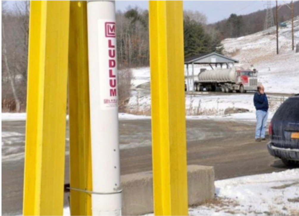
A Ludlum gamma radiation detector
