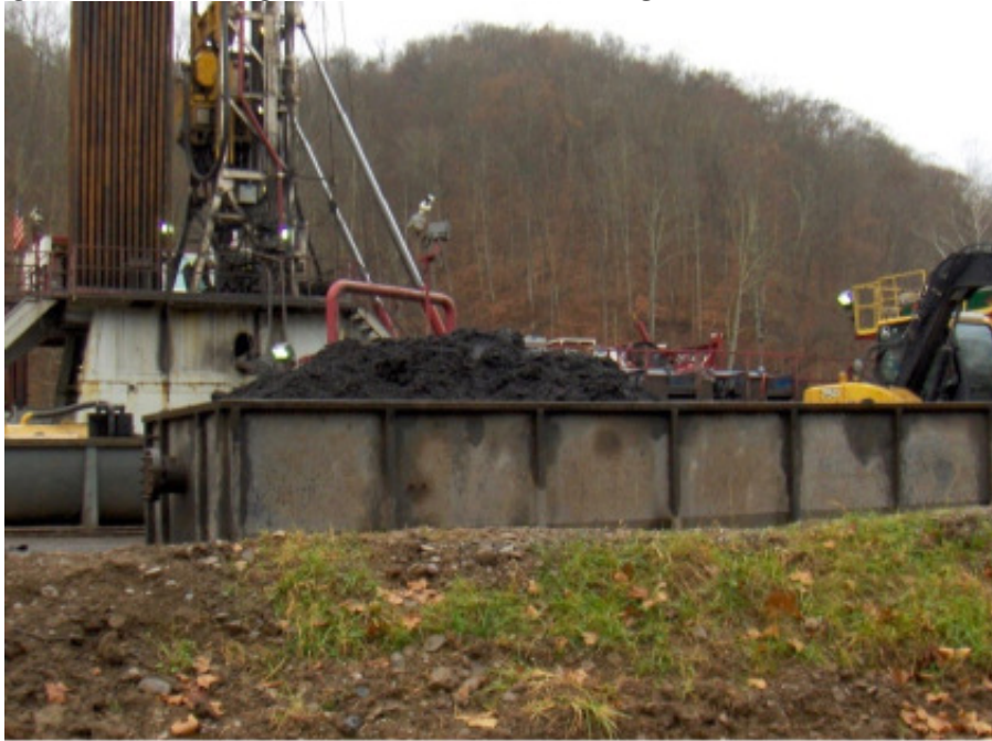
Drill cuttings being prepared for shipment to a landfill.
