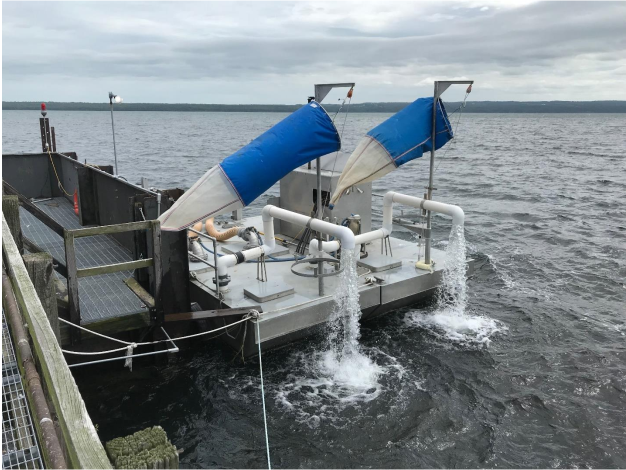
Figure 3-6 Sampling barge in position at south side of Greenidge Generation intake structure in Seneca Lake. Nets are raised because biological sample was not occurring at the time.
