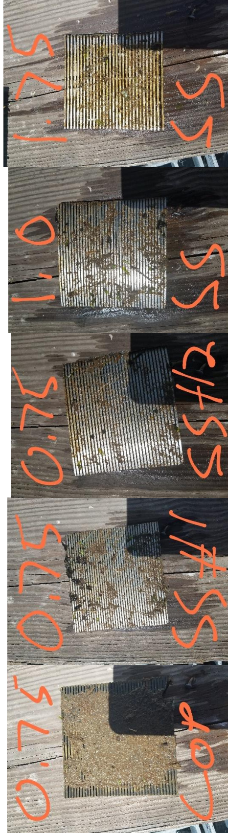
Figure 4-4 Biological fouling of screen coupons after 12 weeks of flow (Event 12). Screen coupons are 0.75 mm slot copper-nickel alloy, 0.75 mm slot stainless steel (#1 and #2), 1.0 mm slot stainless steel, and 1.5 mm slot stainless steel.
