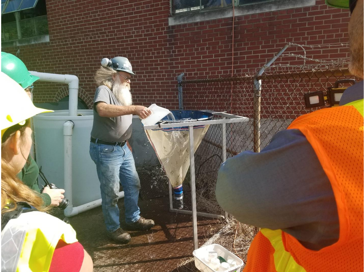
Figure 3-8 Entrainment monitoring equipment (barrel sampler) with net removed for sample extraction.
