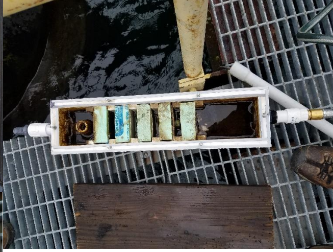
Figure 4-3 Biological fouling of screen coupons after 4 weeks of flow (Event 4). Screen coupons are 0.75 mm slot copper-nickel alloy, 0.75 mm slot stainless steel (#1 and #2), 1.0 mm slot stainless steel, and 1.5 mm slot stainless steel. Bottom photo is the flow-through chamber used to hold the screen coupons in order of decreasing slot width.
