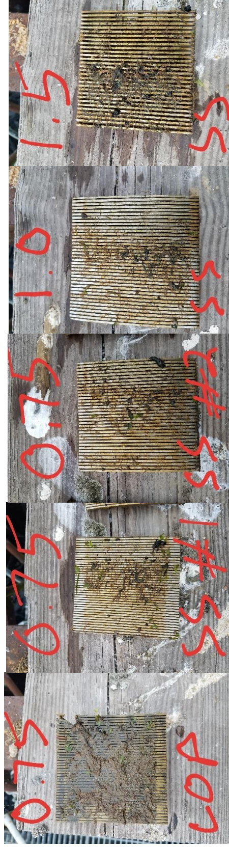
Figure 4-5 Biological fouling of screen coupons after 24 weeks of flow (Event 24). Screen coupons are 0.75 mm slot copper-nickel alloy, 0.75 mm slot stainless steel (#1 and #2), 1.0 mm slot stainless steel, and 1.5 mm slot stainless steel.
