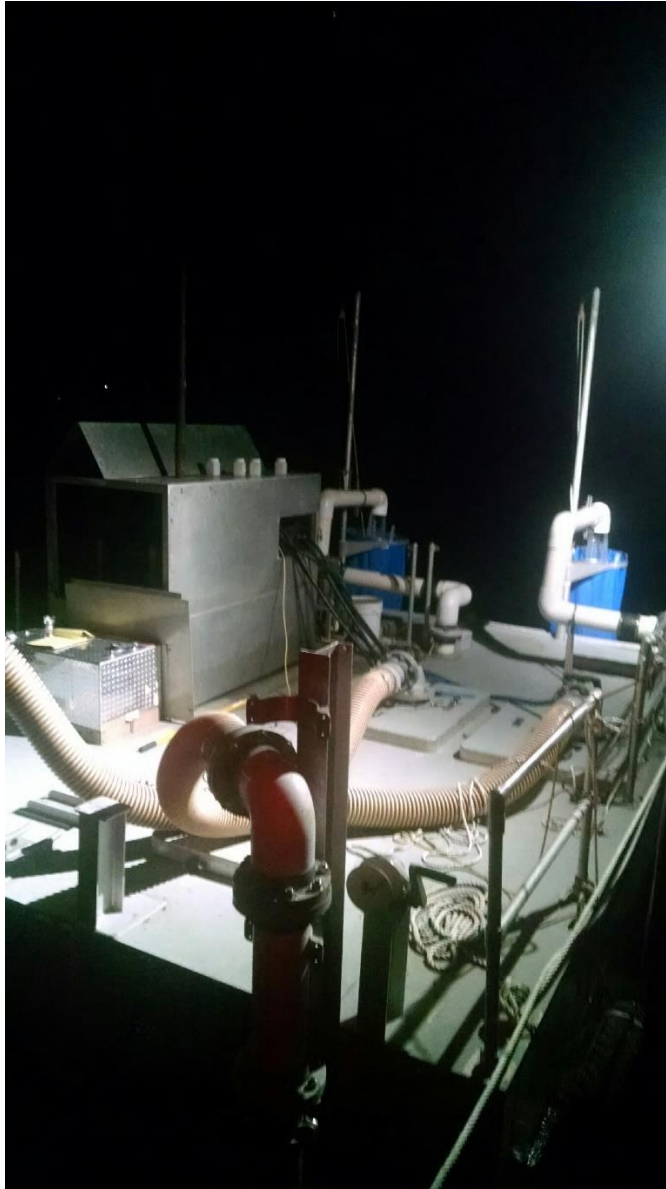
Figure 3-9 Biological sampling of the flow through CWWS screens during nighttime. Nets are positioned to receive the flow and capture entrainable organisms.
