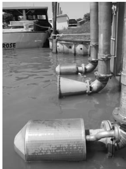
Figure 3-4 Two test screens (near and far), with control intake (mid) used in EPRI wedgewire screen testing.
