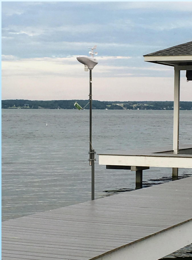
Experimental data logger with water temperature and dissolved oxygen sensor Solar powered (not in picture to left)
