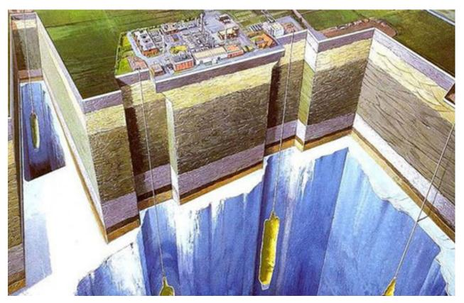
A Salt Cavern Underground Natural Gas Storage Reservoir Configuration. Photo: PB Energy Storage Services Inc.
